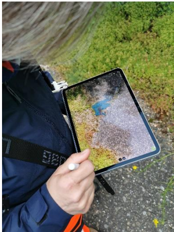
© University Zurich – A field of invasive alien species (here Japanese Knotweed) is first filmed by a drone and labeled on site so that an AI model can later detect them independently on the aerial image (blue area).
