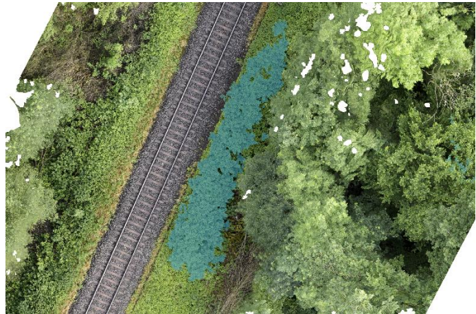
© University Zurich – A field of invasive alien species (here Japanese Knotweed) is first filmed by a drone and labeled on site so that an AI model can later detect them independently on the aerial image (blue area).
